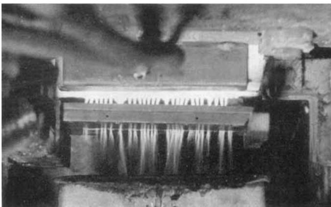
*This photograph of the Owens-Corning glass wool process in operation, taken at an exposure of 1/25 second, gives an impression of the visual appearance of the process. The bottom of the platinum bushing, and the glass above and below the blower chamber, are seen to be incandescent.*
