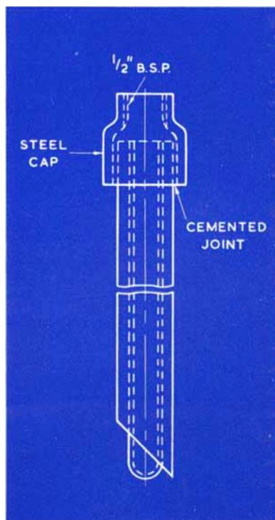
*A composite thermocouple protection tube for continuous immersion. The thin inner tube is of Impervious mullite, sealed into a stout open-ended silicon carbide outer tube*
