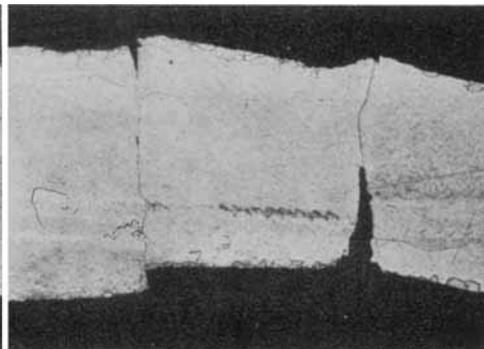
Fig. 5 Section of 13 per cent rhodium-platinum alloy wire after failure in service  $\times 120$
