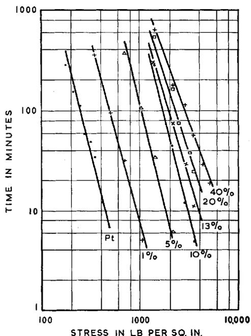
Fig. 1 Stress-to-rupture tests on rhodium-platinum alloys at 1400°C
