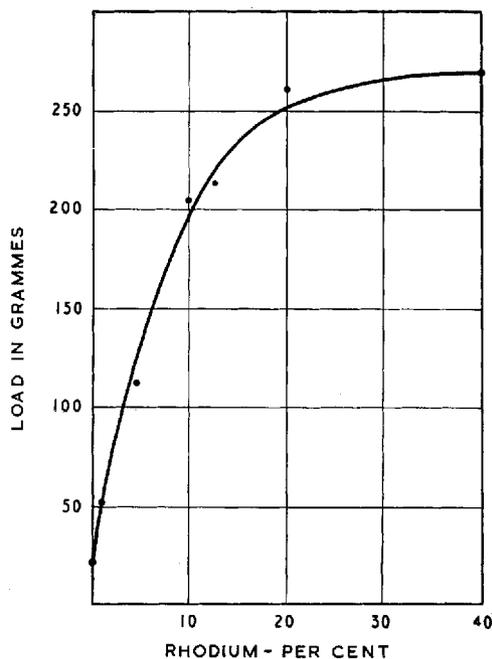
Fig. 2 Load-to-rupture in 250 minutes for rhodium-platinum alloy wires
