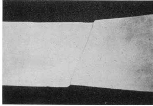
Fig. 3 Section of pure platinum wire after stressing at 1400°C, showing sliding at grain boundary  $\times 120$
