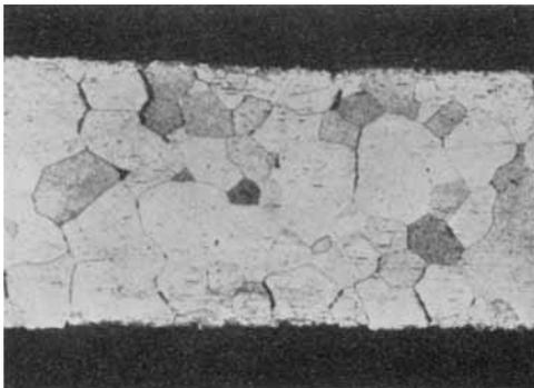
Fig. 4 Section of 5 per cent rhodium-platinum alloy wire after prolonged stressing at 1400°C  $\times 120$
