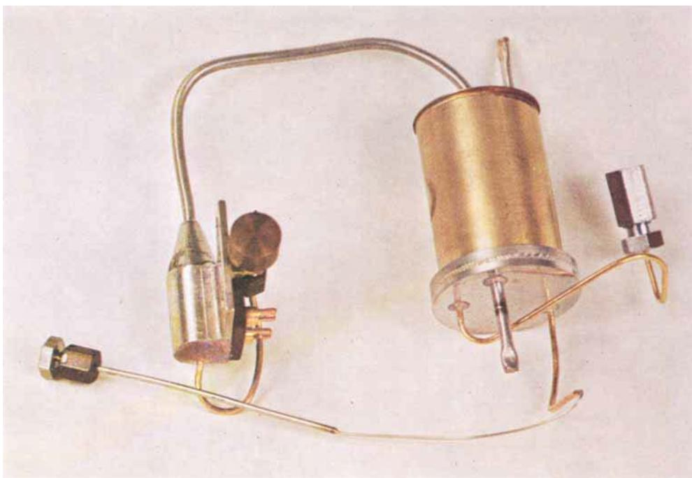
*The palladium-silver diffusion tubes which form the hydrogen separator are contained in the large cylindrical component. Hydrogen and gaseous products pass from the gas chromatograph along the tube at the bottom of the figure to the separator and from here hydrogen is discharged through the device on the left while the products for analysis are lead through an outlet tube to the mass spectrometer connector on the right*
