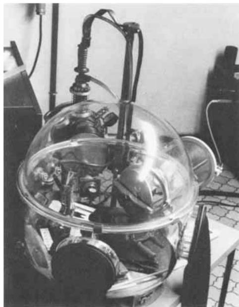
*Fig. 1 Samples for examination were produced from alkali metals and platinum group metals of 99 and 99.9 atomic per cent purity, respectively. This argon filled glove box was used both for the preparation of arc melted samples and to enable the constituent elements to be sealed into tubes or cylinders prior to the reaction processes*
