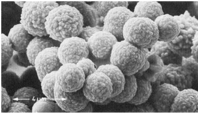
Fig. 5 This powder consists of spherical particles with lower agglomeration than the powder shown in Figure 4, but it has a considerable degree of surface roughness. Although an improvement over previously illustrated material, it remains unsatisfactory for MLCC applications
