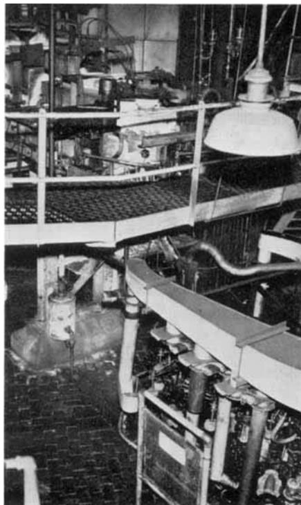
*Platinum thermocouple assemblies installed by Honeywell Controls Ltd. at the Greenford works of Rockware Glass Ltd. are designed for instantaneous temperature measurement of flowing glass in severe conditions*
