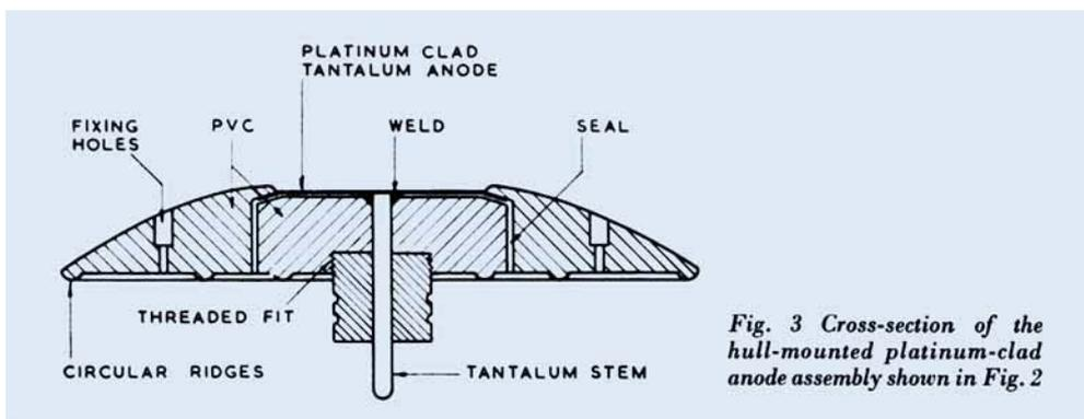
Fig. 3 Cross-section of the hull-mounted platinum-clad anode assembly shown in Fig. 2
