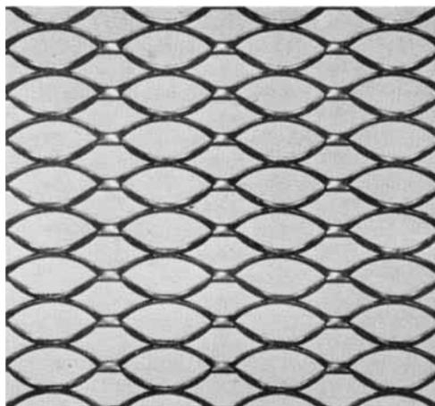
Fig. 1 Detail of expanded platinum-clad tantalum anode. Thickness of platinum is 0.00025 inch. (Metals and Controls Corporation)
