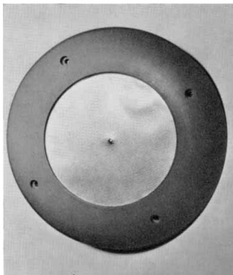
Fig. 2 A hull-mounted platinum-clad tantalum anode. The embossing of the surface assists liberation of gaseous products formed during electrolysis. (Metals and Controls Corporation)
