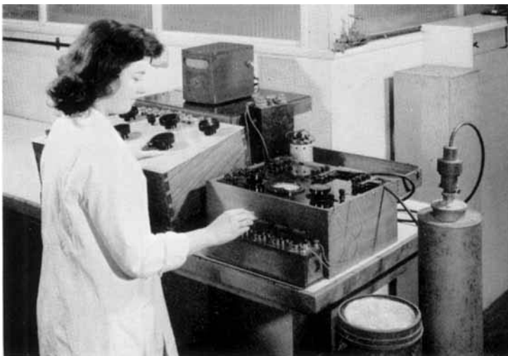
A physicist in the Johnson Matthey Process Control Laboratory determining the temperature coefficient of resistance between 0° and 100°C of the Thermopure platinum produced specially for resistance thermometry.
