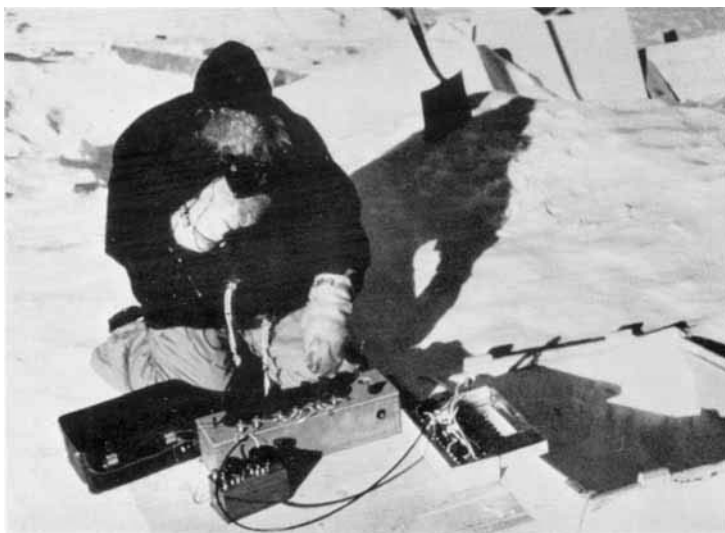
Dr. H. Lister, the glaciologist of the Trans-Antarctic Expedition led by Sir Vivian Fuchs, using a platinum resistance thermometer to measure temperatures from -15° to -60°C at different depths in the ice. The photograph was taken at the advance base "South Ice", 4,400 feet above sea level and 300 miles south of Shackleton on the Weddell Sea.
