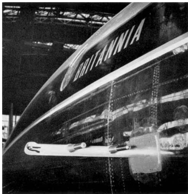
A resistance thermometer by Sangamo Weston Limited, to measure air temperature for speed correction, may be seen behind the shield at the end of the spar on the port side of the Bristol Britannia. The spar also carries two ice detectors.
