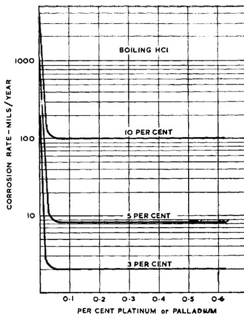
*Effect of platinum and palladium additions to titanium on rate of corrosion in various concentrations of boiling hydrochloric acid*
