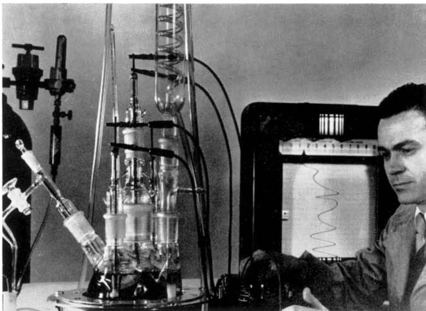
*Electrochemical apparatus used in the Metals Research Laboratories of Union Carbide Metals Company in obtaining data on the dissolution of metals by plotting anodic and cathodic polarisation curves. The electrochemical data show that small additions of noble metals to titanium bring about passivity and a marked decrease in the rate of corrosion*
