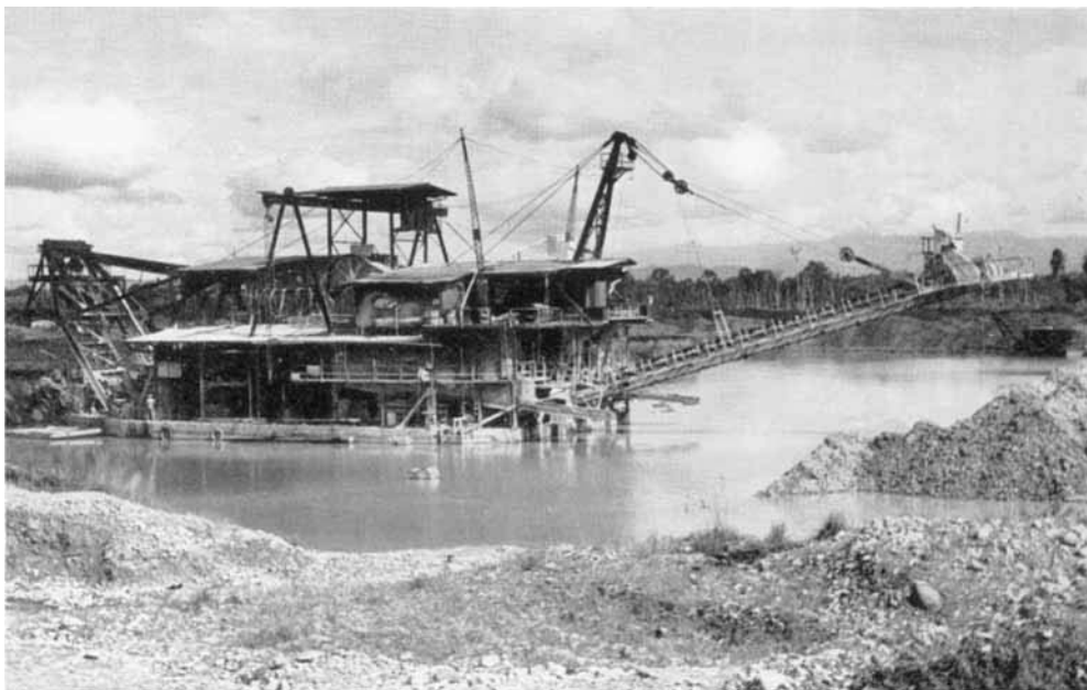
One of the modern mechanical dredges operated by the Compania Minera Choco Pacifico in the main platinum area now being worked near the San Juan river in Colombia
