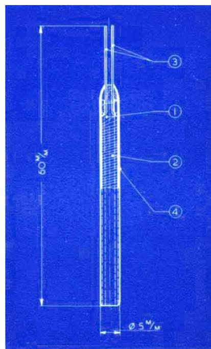
*The construction of the platinum resistance thermometer, type W85*
