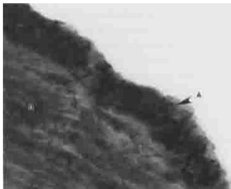
**Fig. 3** TEM Bright field image of a palladium coated particle; 1 cm represents  $0.08 \mu\text{m}$
