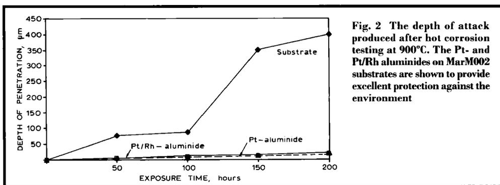
Fig. 2 The depth of attack produced after hot corrosion testing at 900°C. The Pt- and Pt/Rh aluminides on MarM002 substrates are shown to provide excellent protection against the environment
