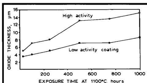
**Fig. 1** Oxide thickness measurements taken from the high and low activity coatings on alloy MarM002 substrates, indicating the superior scale for the low activity coating. MarM002 is a nickel-based alloy, containing small additions of titanium and hafnium. It is used extensively in powder form to repair turbine blades damaged by oxidation and hot corrosion
