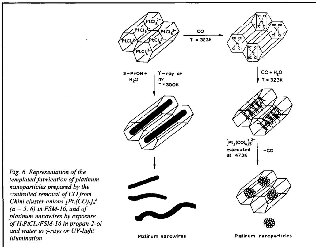
Fig. 6 Representation of the templated fabrication of platinum nanoparticles prepared by the controlled removal of CO from Chini cluster anions [Pt<sub>3</sub>(CO)<sub>6</sub>]<sup>2-</sup> (n = 5, 6) in FSM-16, and of platinum nanowires by exposure of H<sub>2</sub>PtCl<sub>6</sub>/FSM-16 in propan-2-ol and water to γ-rays or UV-light illumination
