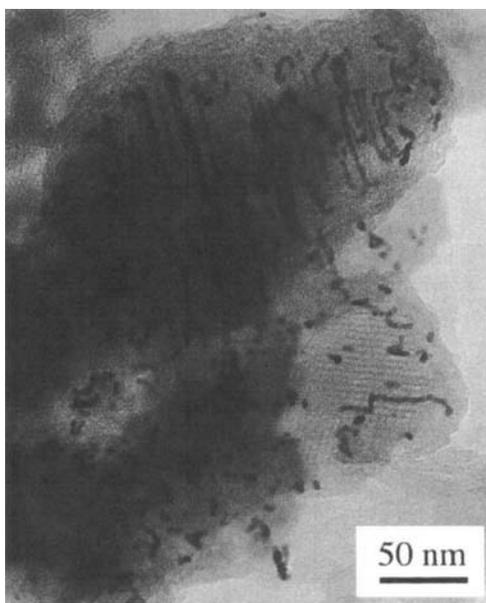
*Fig. 7 TEM of platinum nanowires in FSM-16 prepared by the reduction of  $H_2PtCl_6/FSM-16$  with propan-2-ol and water by  $\gamma$ -ray irradiation at 300 K for 5 hours. The nanostructured wires (3 nm  $\times$  50–200 nm long) are clearly aligned in the ordered channels of FSM-16 (28 Å)*
