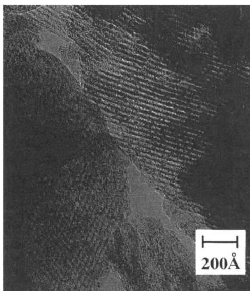
Fig. 5 TEM of platinum nanoparticles (diameter 15 to 20 Å) prepared by controlled removal of CO at 573 K for 5 hours from Chini cluster anions, [Pt<sub>15</sub>(CO)<sub>30</sub>]<sup>2-</sup>, synthesised in FSM-16. The particles are uniformly aligned in the ordered FSM-16 (28 Å) channels
