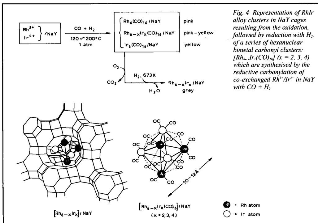
Fig. 4 Representation of Rh/Ir alloy clusters in NaY cages resulting from the oxidation, followed by reduction with H<sub>2</sub>, of a series of hexanuclear bimetal carbonyl clusters: [Rh<sub>6-x</sub>Ir<sub>x</sub>(CO)<sub>16</sub>] (x = 2, 3, 4) which are synthesised by the reductive carbonylation of co-exchanged Rh<sup>3+</sup>/Ir<sup>4+</sup> in NaY with CO + H<sub>2</sub>.
