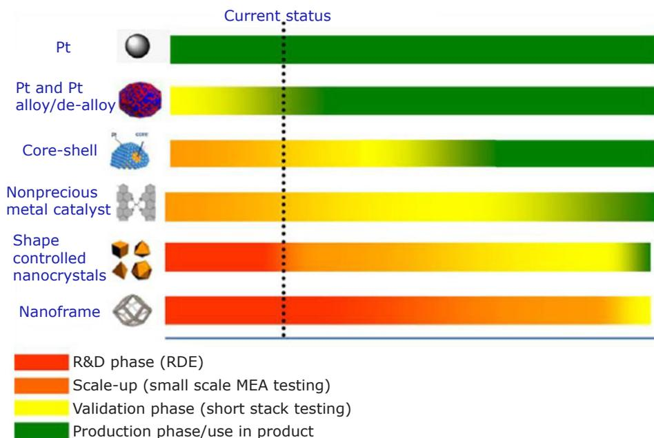
Fig. 1. Timeline giving a general ranking of technology readiness for each catalyst family for fuel cells. R&D = research and development, MEA = membrane electrode assembly. Copyright 2021 Elsevier
